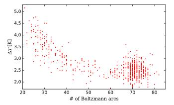
**Figure 5.** Error in temperature determination as a function of the number of successful fits of Boltzmann distributions of single vibrational transitions.
