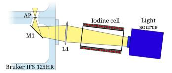
Figure 2. Schematic setup of the experiment. Uncollimated light from the source passes through the iodine cell and is focused by lens L1 on to the FTS entrance aperture AP. Note that fold mirror M1 and the entrance aperture are inside the Bruker IFS 125HR.
