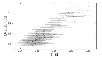
**Figure 8.** Effective RV/wavelength shift as a function of temperature during periods where the heating is turned off.
