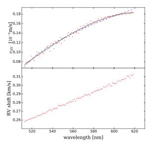
Figure 7. Top row: Wavelength dependence of the RV precision  $\sigma_{RV}$  for the combined spectra in bins of width 1 nm. The dashed blue line represents a square root law fit, while the solid black line represents a logarithm multiplied with a linear function (equation 26). Second row: Total effective RV/wavelength shift as a function of wavelength.
