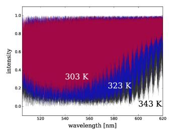
**Figure 4.** Total spectrum for three different cell temperatures (303, 323, and 343 K). At 323 K, a large part of the spectrum is already saturated.
