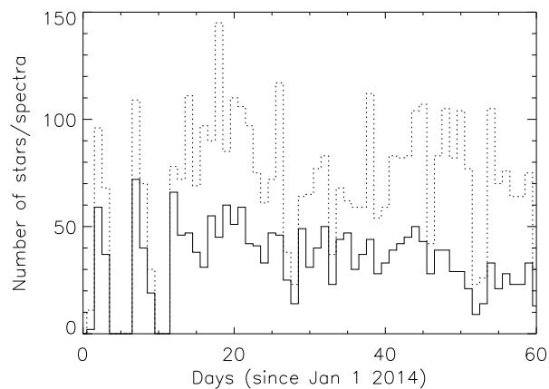
**Fig. 8** TIGRE efficiency as measured in terms of obtained spectra per night (dotted histogram) and stars observed per night (solid histogram); as can be seen, the system has no problem observing more than 70 different objects per night.
