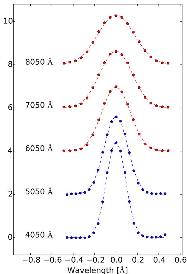
**Fig. 5** Some examples of TIGRE calibration line profiles covering the whole spectral range. While the absolute width of the spectral lines increases with wavelength, the relative width decreases, leading to a slightly increasing spectral resolution with increasing wavelength.
