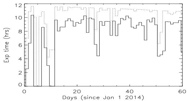
**Fig. 7** TIGRE efficiency as measured in terms of hours of exposure per night (solid histogram) in comparison to total available time (dotted histogram); during good nights the TIGRE system reaches more than 90 % efficiency.
