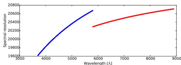
**Fig. 6** TIGRE spectral resolution as determined from ThAr calibration lines in the blue arm (blue curve) and red arm (red curve).
