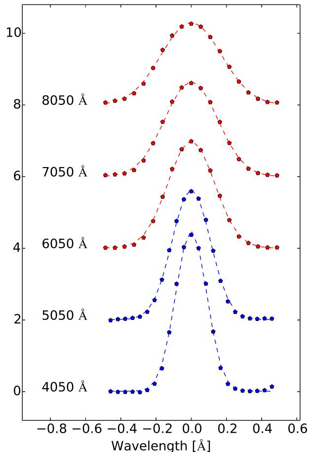
**Fig. 5** Some examples of TIGRE calibration line profiles covering the whole spectral range. While the absolute width of the spectral lines increases with wavelength, the relative width decreases, leading to a slightly increasing spectral resolution with increasing wavelength.
