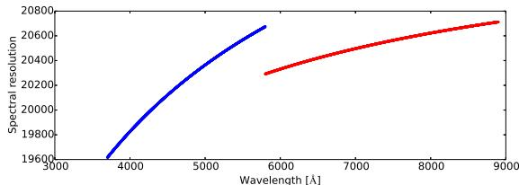
**Fig. 6** TIGRE spectral resolution as determined from ThAr calibration lines in the blue arm (blue curve) and red arm (red curve).
