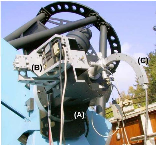
**Fig. 2** The TIGRE adapter. A: Nasmyth platform of the telescope; B: the adapter with the flanged guiding camera in the foreground; C: Fiber holder with the fiber inside a protective tube.
