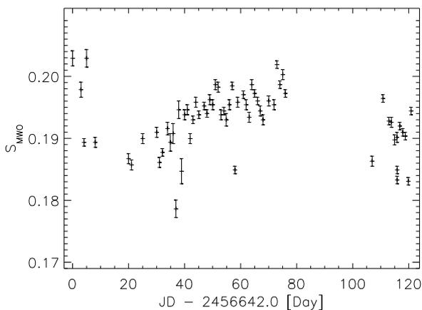
**Fig. 12** S-index vs. time for  $\tau$  Boo; from TIGRE spectra a transformation into the Mount-Wilson S-index scale has been derived. This S-index time series demonstrates the capability of TIGRE to produce densely sampled activity monitoring.
