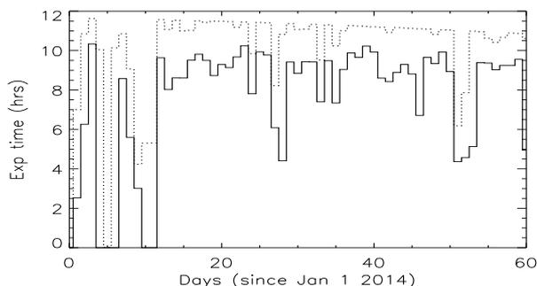
**Fig. 7** TIGRE efficiency as measured in terms of hours of exposure per night (solid histogram) in comparison to total available time (dotted histogram); during good nights the TIGRE system reaches more than 90 % efficiency.
