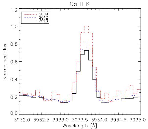
**Fig. 10** TIGRE spectra of the Ca II K line core of 61 Cyg A taken in 2009, 2012, and 2013. Note the decline in the core emission strength with the declining cycle of 61 Cyg A, as well as the much improved spectral quality of the data taken since 2012.
